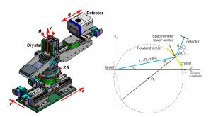
Left: Actual desing of the DuMond spectrometer with the Pilatus 100K-S 2D detector and the dedicated crystal bender on top. Right: Geometry of the DuMond type Spectrometer
