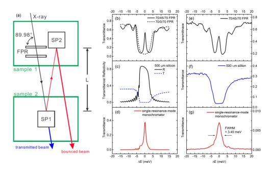
(a) The scheme of the IM consisting of a FPR and DCM (SP1 and SP2), the simulated spectra of (b) the FPR, (c) the SP1 or SP2 and (d) the IM and the measured results of (e) the FPR, (f) the SP1 and (g) the IM.
