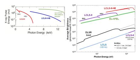
Calculated energy per pulse (left) and average brightness (right) for LCLS-II and proposed LCLS-II-HE, including future X-ray facilities: the European XFEL and diffraction-limited storage rings (DLSRs).
