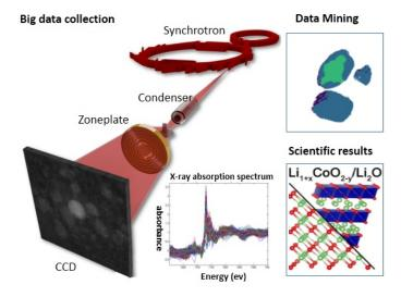
**Big Data collection:** Nanoscale X-ray spectro-microscopy technique (beamline 6-2C of SSRL) collects spatially resolved x-ray absorption spectra at very fast data rate. **Data Mining:** Advanced data mining approach developed in this work searches through over 10 million spectra and identified two particles with unanticipated chemical fingerprints. **Scientific results:** These two particles are attributed to two different unwanted side reactions.
