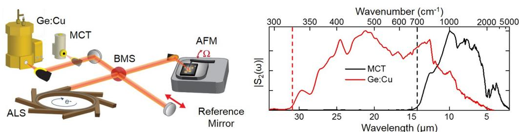
(A) Schematic of SINS experimental configuration: beamsplitter (BMS), atomic force microscope (AFM), mercury cadmium telluride (MCT), copper-doped germanium (Ge:Cu). (B) SINS signal on gold with two different detectors, illustrating the broad spectral range.
