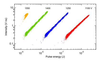
The responsivity of the MCP detector compared with the LCLS upstream gas detector. The anode voltage was varied from 1100 to 1550 V.
