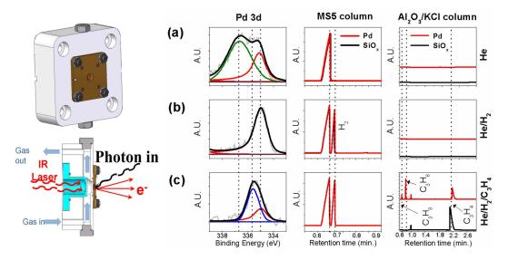
Pd 3d XP spectra and gas chromatography traces (VARIAN  $\mu$ GC 4900) using a mol sieve MS5 column (VARIAN CP740148) and Al<sub>2</sub>O<sub>3</sub>/KCl column(AGILENT 494001440) : a) He, b) He/H<sub>2</sub>, and c) He/H<sub>2</sub>/C<sub>3</sub>H<sub>4</sub> gas mixtures.
