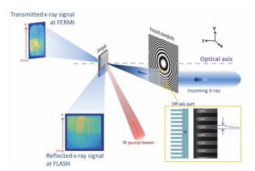
Schematic diagram of the setup concept. At FLASH the reflected probe x-ray was recorded. At FERMI, the transmitted signal was collected downstream of the sample. In both cases, the time information is encoded in spatial coordinates in the recorded images.
