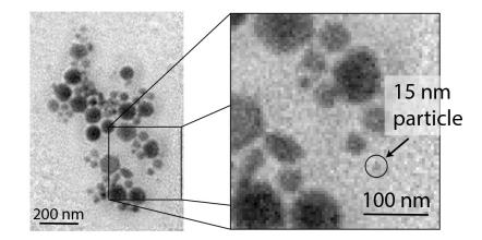
Ptychographic reconstruction of a cluster of nanoparticles made of gold, platinum, and palladium deposited on a  $Si_3N_4$  membrane. The smallest particles that can resolved are about 15 nm in size. For details see [5].
