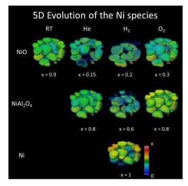
Phase distribution volumes of NiO,  $NiAl_2O_4$  and Ni as obtained from the Rietveld analysis of the 3D-XRD-CT datasets collected at the four different operating conditions.
