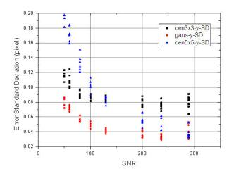
The effect of SNR on position estimation error standard deviation. Three algorithms,  $3 \times 3$  centroid,  $5 \times 5$  centroid and 2-D Gaussian fitting are compared. The SD decreases when SNR increases. 2-D Gaussian fitting gives the more accurate position than the other two algorithms.
