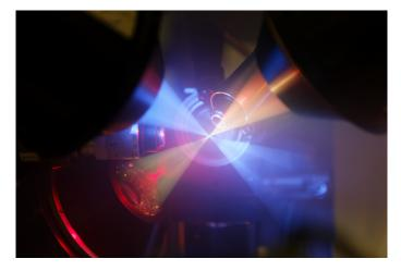
The new offline microspectrophotometer of the ID29S-Cryobench laboratory at the ESRF. Three blue, green and red LEDs highlight the intersection of the focal volumes of the three optical objectives.
