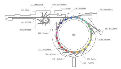
Schematic layout of the MAX IV facility showing the linac together with the 1.5 GeV and 3 GeV storage rings and the beamlines presently in operation or building.
